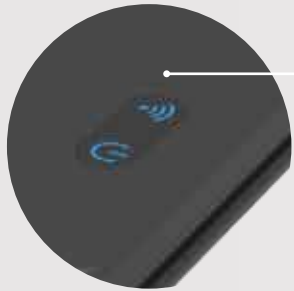
LED indicators Wi-Fi and Power
