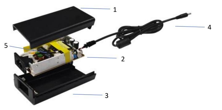
Separate 11: Pry open Part 1 and Part 3 to take out the Part 2.
