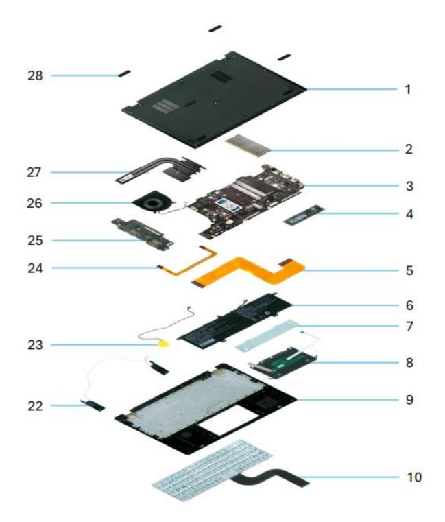
Separate 7: Unscrew all screws(5pcs) and unplug the keyboard cable to take out the Part 8.
