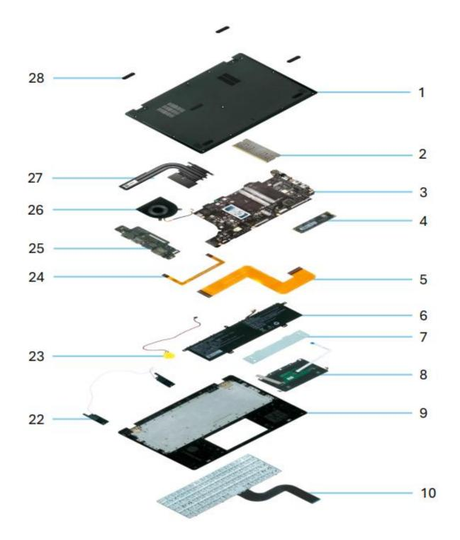
Separate 8: Remove Part 9, unscrew all screws(3pcs) to take out the Part 25.
