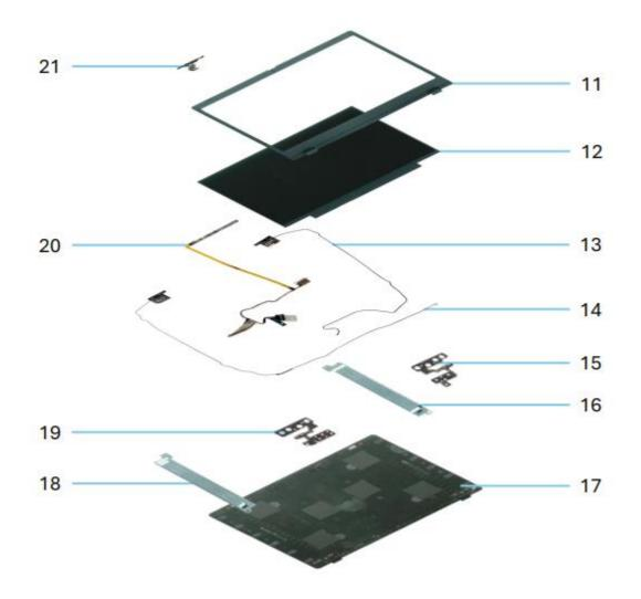
Separate 9: Remove Part 11, unscrew all screws(8pcs) on Part 17 to take out the Part 12.
