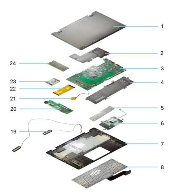
Separate 6: Unscrew all screws(8pcs) and unplug the cables to take out the Part 3 and Part 20.
