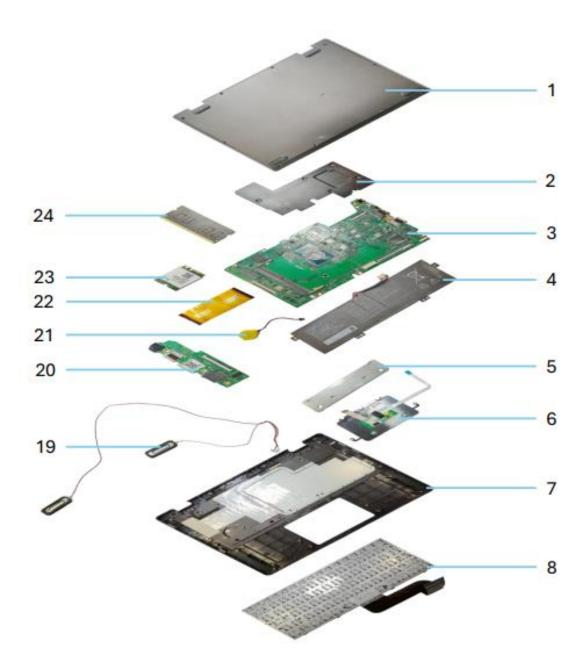
Separate 7: Unscrew all screws(2pcs) on part 7 to take out the Part 8.
