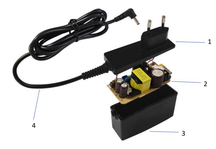
Separate 11: Pry open Part 1 and Part 3 to take out the Part 2.
