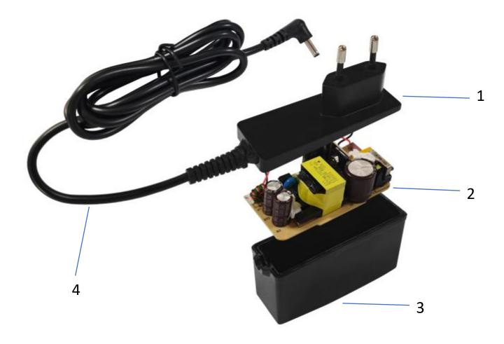
Separate 12: Pry open Part 1 and Part 3 to take out the Part 4.
